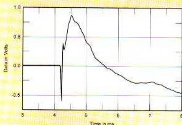
Fig.8 Vienna Acoustics Mahler, step response at 50° (5ms time window, 30kHz bandwidth).
